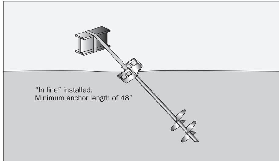
Failure occurs when the stresses exceed the soil shear strength. The geometry of the failure surface varies based on the critical depth of the anchor. Ground anchors with an embedment depth less than the critical depth to anchor base width ratio  $((D/B)_{cr})$  respond as a shallow foundation. Ground anchors with a depth greater than  $(D/B)_{cr}$  respond as a deep foundation.
