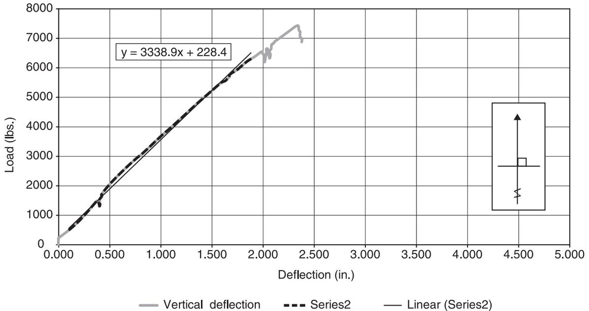
Figure 7-6. Typical response for an axially loaded anchor.
