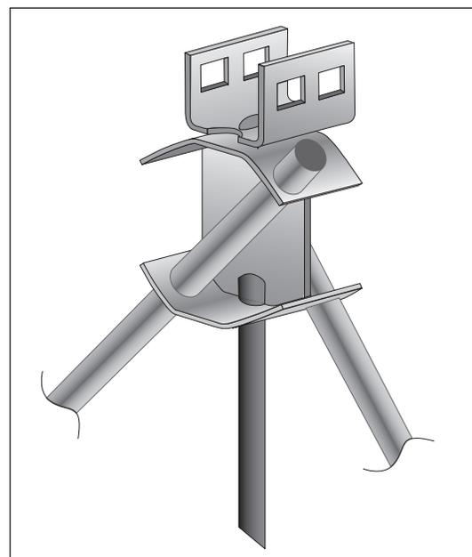
Figure 7-1. Cross drive anchor. (Courtesy of Tie Down Engineering)
