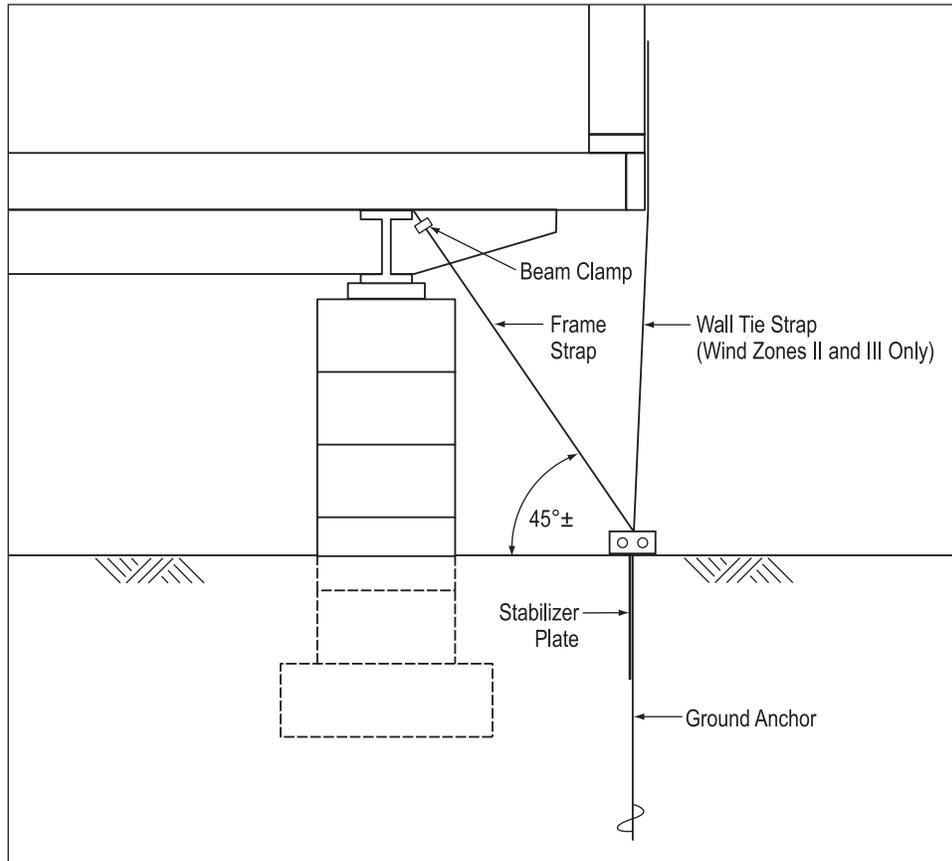
Figure 7-4. Typical ground anchor installation.
